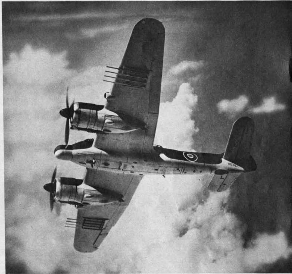
Beaufighter X (above and below) has added a snoutlike radome and a long dorsal fin to its basic airframe, giving it one of the war's most irregular plane shapes. Radome extends the Beau's short nose, while dorsal fin makes recognition easier.
